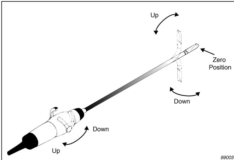
Fig. 4. Movement of the Types 8666 and 8666-RF's flexible tip. Up and down
