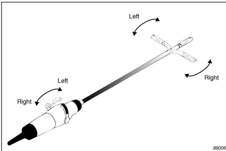
Fig. 5. Movement of the Types 8666 and 8666-RF's flexible tip. Right and left
