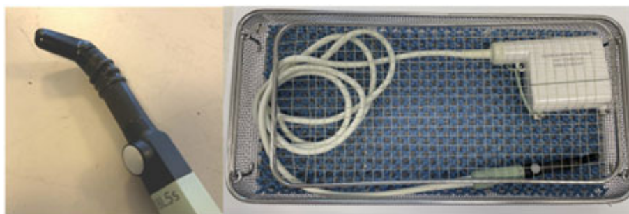
Figure 1-1. X18L5s (9009) with articulation joint in neutral position and secured in a washer-disinfector tray
