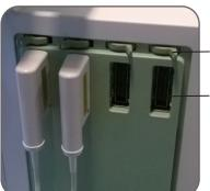
Flip lever left to lock, and right to unlock
