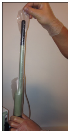
Figure 10. Putting on the inner cover.
