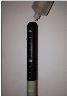
Figure 9. Moistening the transducer with water.
