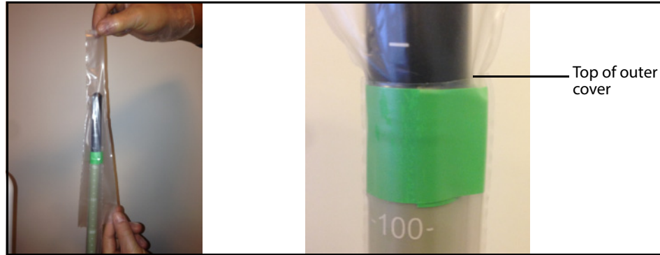
Figure 14. Pulling the outer cover on to cover the tape completely.
