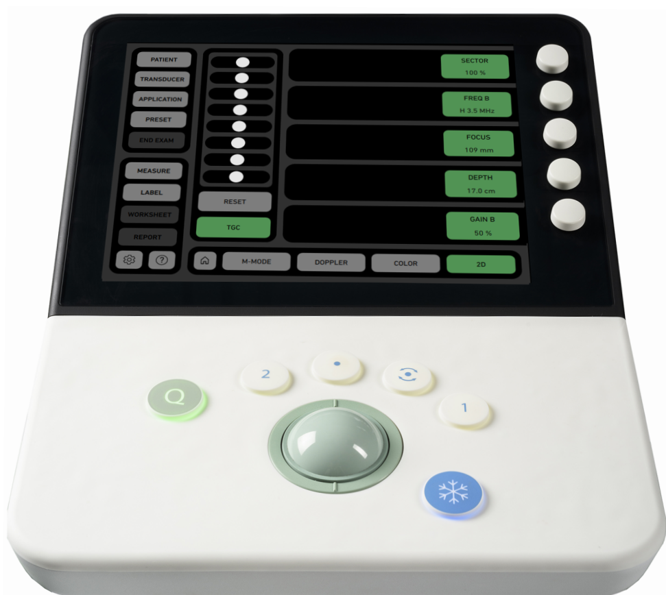
Figure 2-4. The control panel and touch screen.
