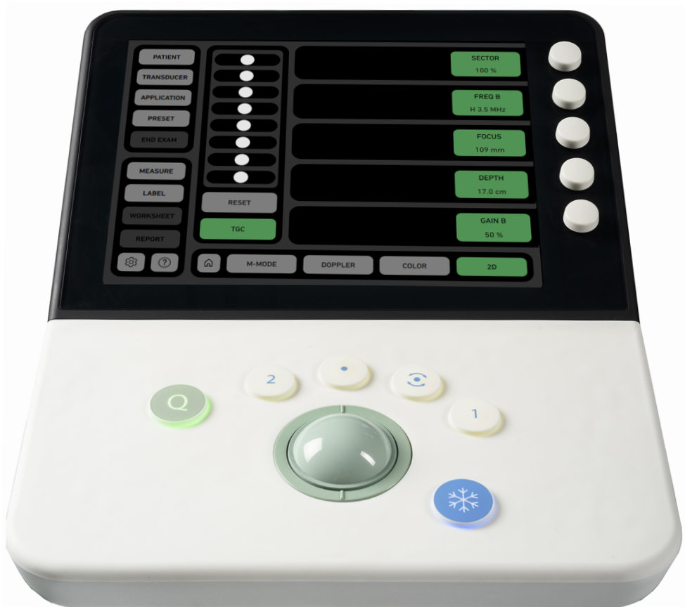
Figure 2-4. The control panel and touch screen.
