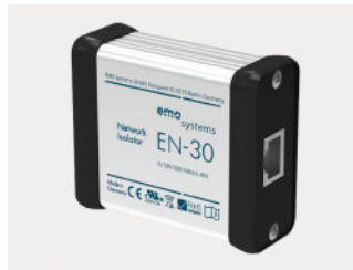
Figure 11-9. Network isolator for the connection to the Kick system.
