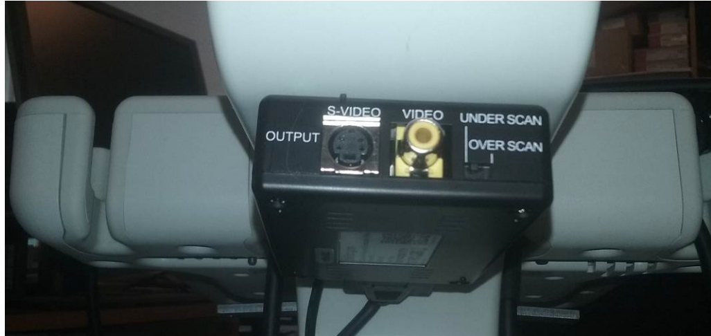
Figure 11-6. Connectors on the DVI/VGA to S-video Converter Kit (UA1311)
