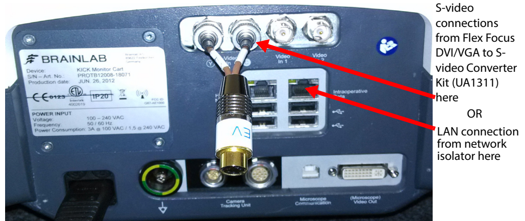
Figure 11-8. Brainlab connections (Kick™ Image Guided Surgery).
