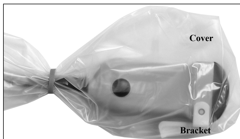
Figure 6. 8823 with reusable bracket and transducer cover.
