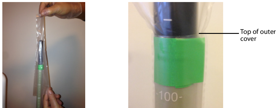
Figure 13. Pulling the outer cover on to cover the tape completely.
