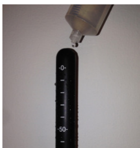
Figure 8. Moistening the transducer with water.
