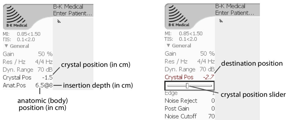
Figure 5. Position of the 2052 transducer crystal.
